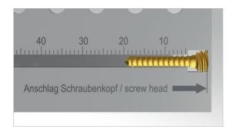
Insertion of the screw into the drilled core hole with the screw driver in the set.
